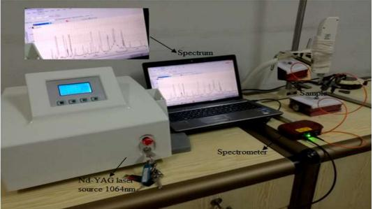
Figure 2-Laser-induced breakdown spectroscopy system
