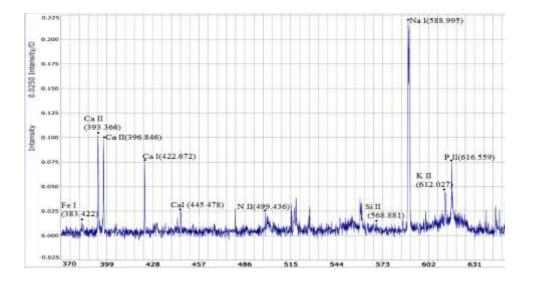
Figure 6-LIBS spectra recorded from Garmah soil.
