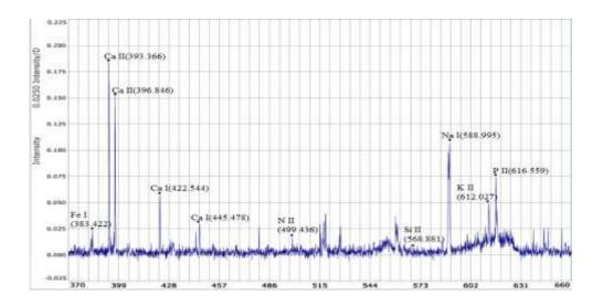
Figure 7-LIBS spectra recorded from Fallujah soil.
