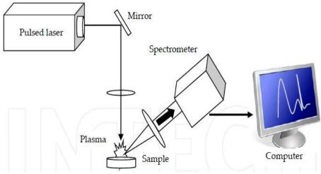
Figure 3-A schematic diagram of the LIBS system.
