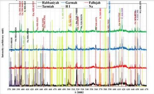
Figure 9-The LIBS emission spectra recorded of the different samples of soils.
