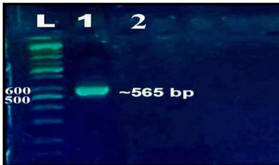
Figure 4- Agarose gel electrophoresis of PCR product the band size ~565 bp. The product was electrophoresis on 2% L: DNA ladder (100), lane (1) Trichoderma isolate, lane (2) negative control sample (no DNA template).
