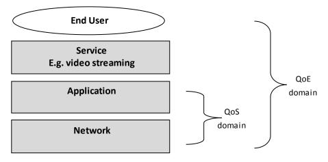
Figure 1- QoS and QoE architecture [6]
