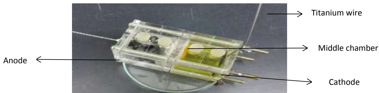
Figure 1- Show the Design of MDC Three-chamber MDC used for desalination.
