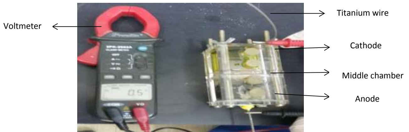
Figure 2- Shows voltmeter in the MDC for Bacillus spp. produce voltage to reduce salinity across circuit.
