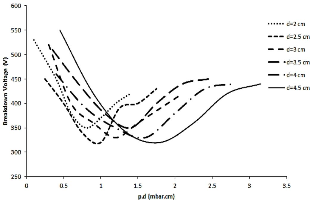
**Figure 8-** Paschen curves presents the breakdown voltage VB as a function of p.d using 2:1 argon to oxygen ratio at different d from 2.5 to 7.5cm.
