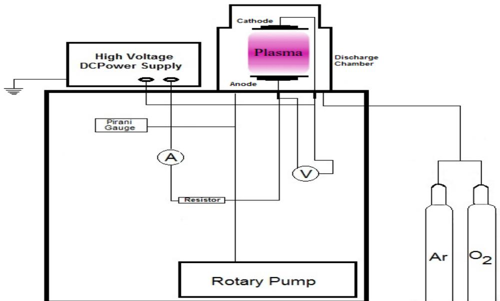
**Figure 1**-Schematic diagram of the sputtering system.
