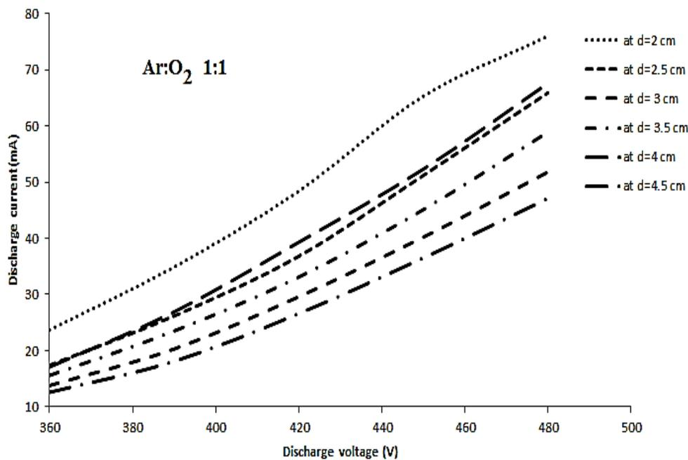
**Figure 5-** Discharge current-voltage characteristics for  $Ar: O_2$  1:1, at pressure gas of 0.15 mbar with different  $d$  (inter-electrode distance)
