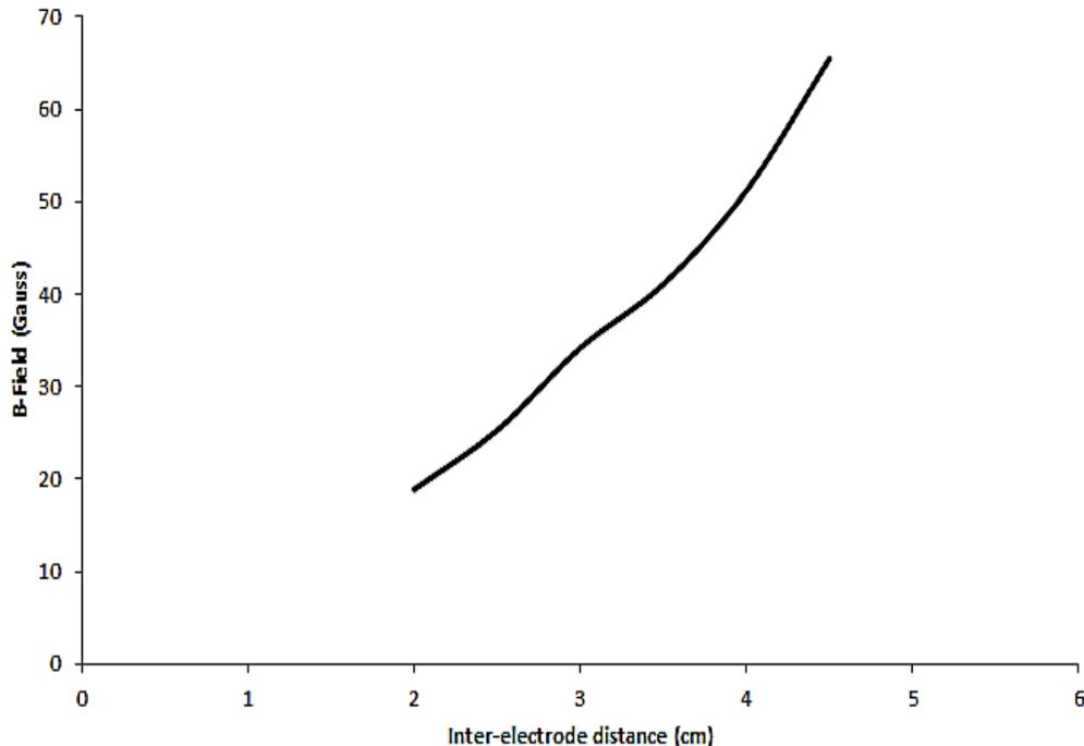
**Figure 9-**The magnetic field intensity as a function of inter-electrode distance.
