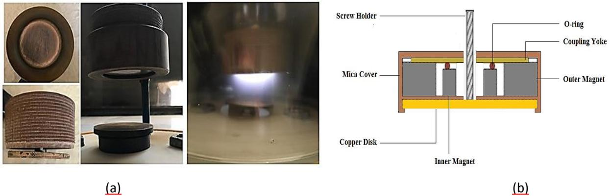
**Figure 2-**shows: (a) Design of discharge electrode used in the work and (b) a photograph of the magnetron at each electrode, and the plasma produced between the two magnetrons.
