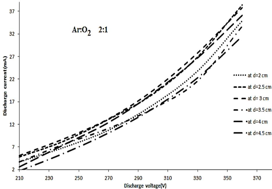
**Figure 6-**Discharge current-voltage characteristics at Ar: O<sub>2</sub> 2:1, at gas pressure of 0.15 mbar with different  $d$  (inter-electrode distance)
