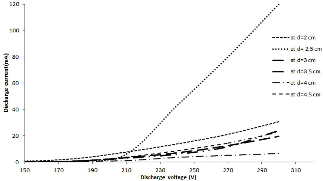
**Figure 3-**the discharge current as a function of discharge voltage (I-V characteristics) at different inter-electrode distances from 2 to 4.5cm at a gas pressure of 0.15 mbar
