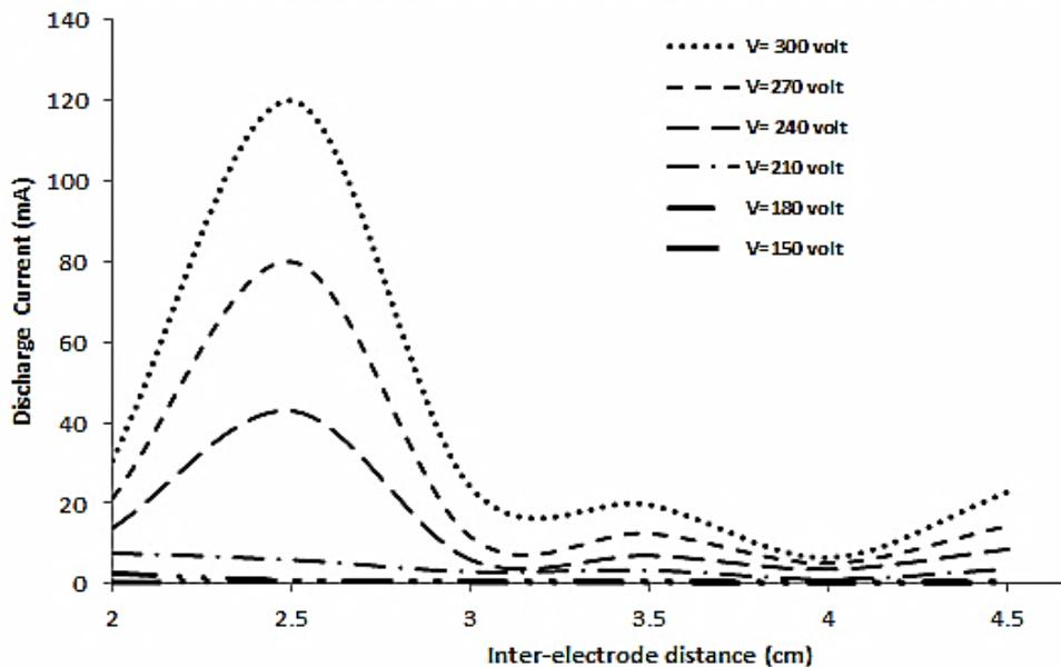
**Figure 4-**The discharge current  $I$  as a function of inter-electrode distance  $d$  with different discharge voltages  $V$ .
