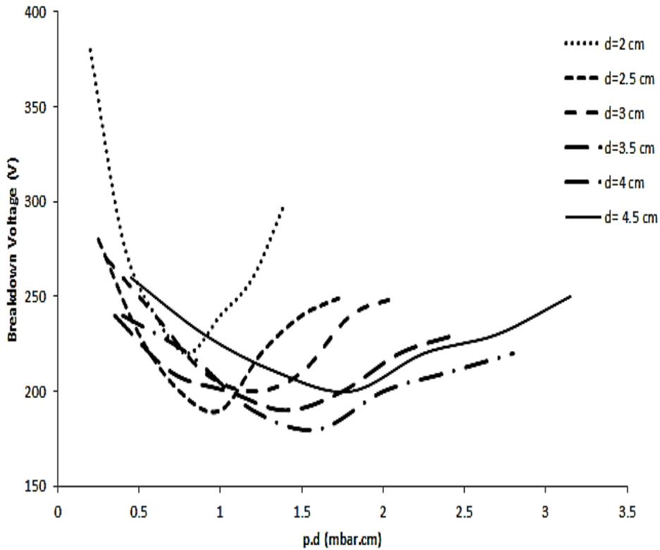
**Figure7-** Paschen curves gives the breakdown voltage as a function of inter-electrode distance using argon gas discharge at different d from 2 to 4.5cm.
