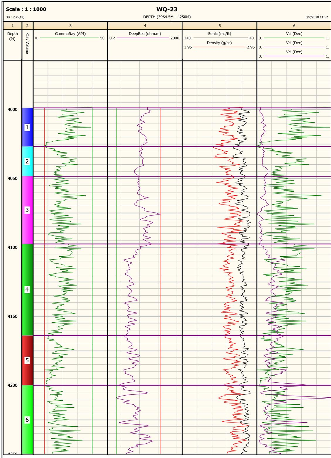
Figure 30- Depth plot of well logs, the distributions of the flow units of WQ-23.
