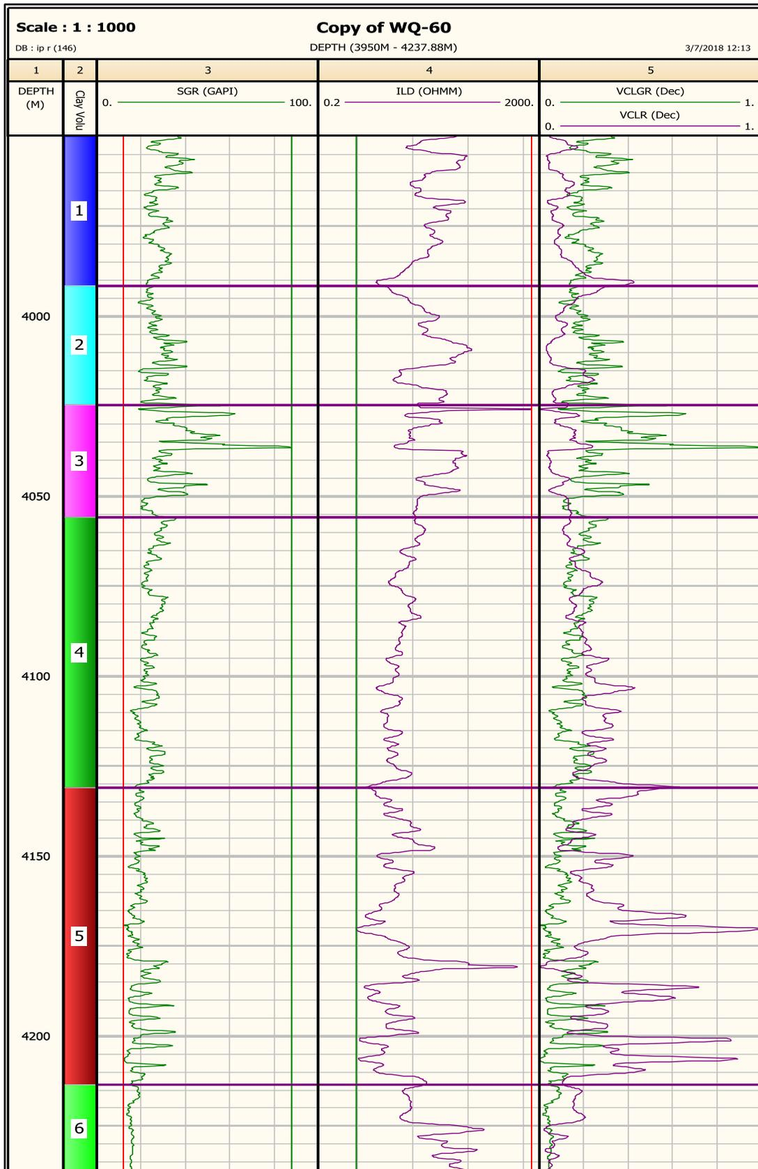
**Figure 31-** Depth plot of well logs, the distributions of the flow units of WQ-60.
