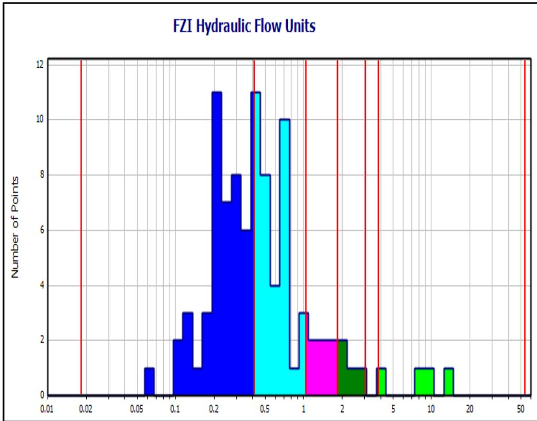
Figure 12- Histogram hydraulic flow units of WQ-60.
