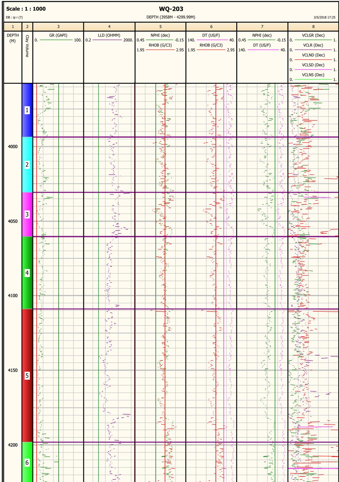
Figure 29- Depth plot of well logs, the distributions of the flow units of WQ-203.
