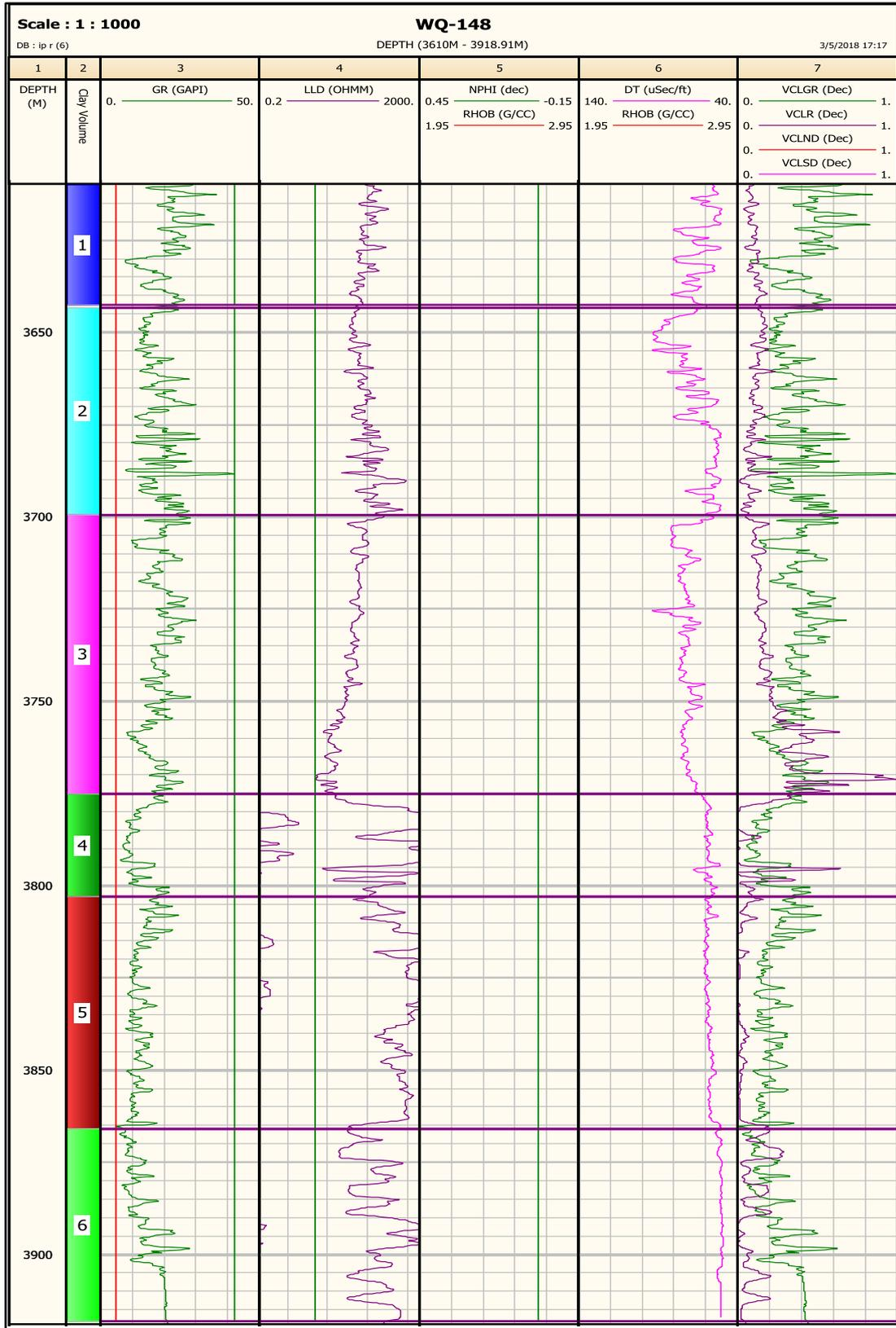
Figure 28- Depth plot of well logs, the distributions of the flow units of WQ-148.
