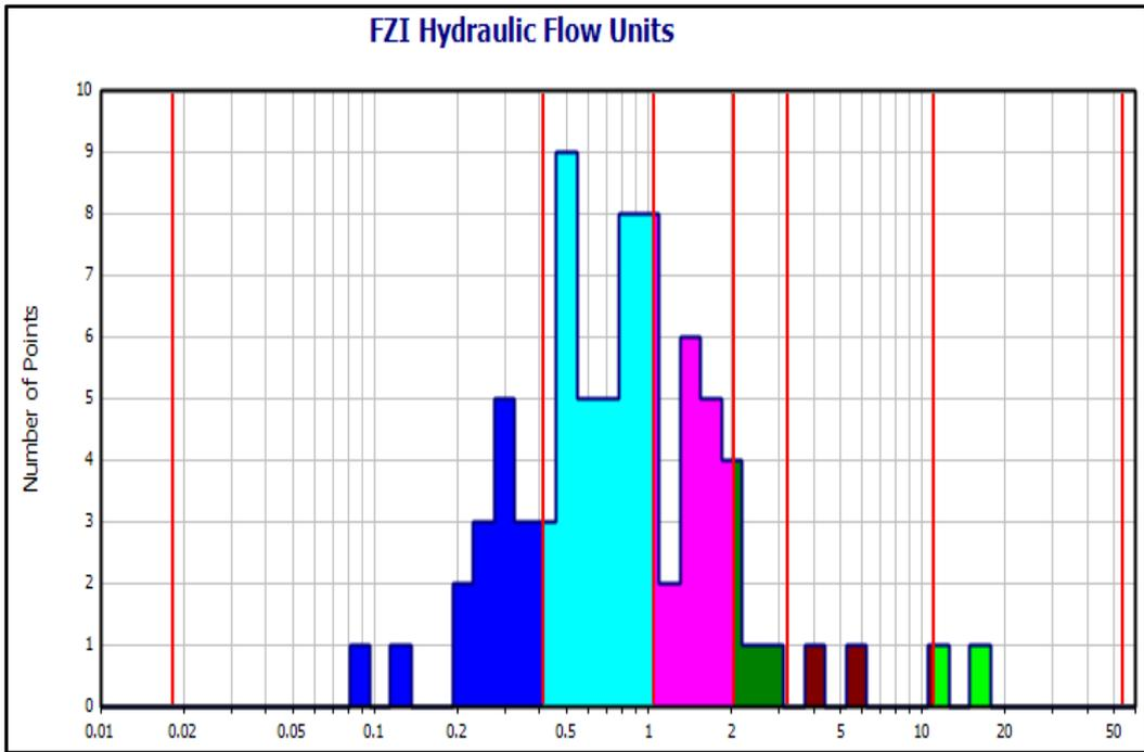
Figure 6- Histogram hydraulic flow units of WQ-203.
