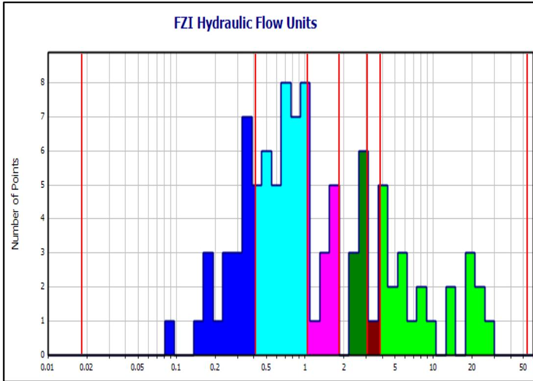
Figure 24- Histogram hydraulic flow units of WQ-23.
