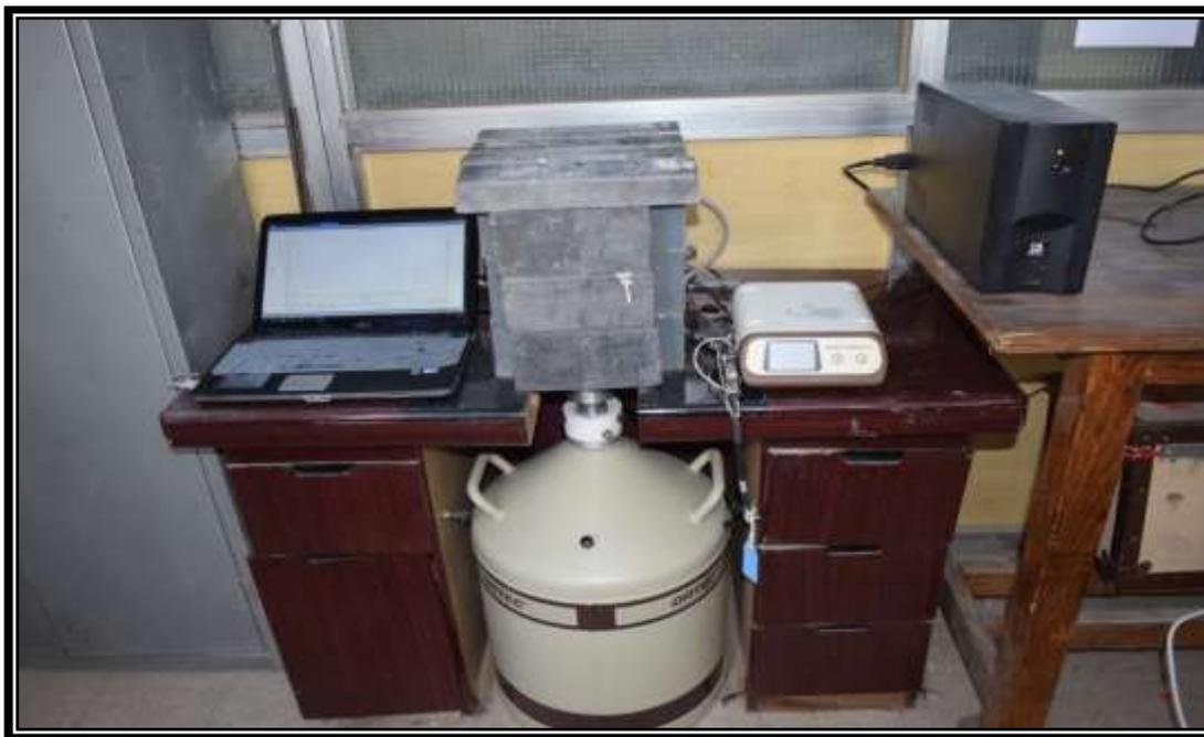
Figure 1-(HPGe) detector system.
