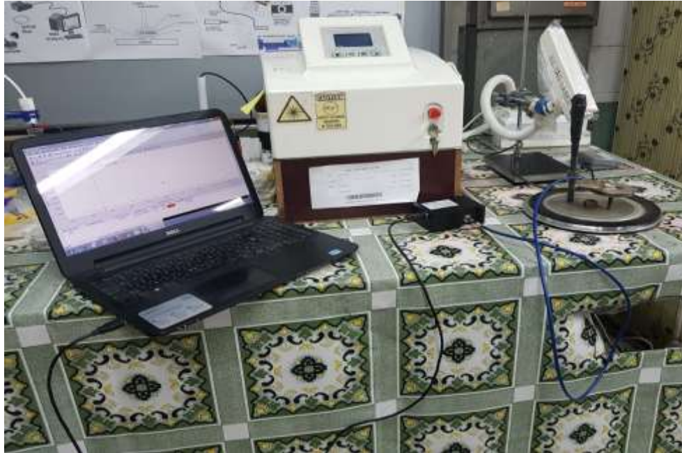
Figure 1- Schematic diagram of the experimental LIBS set-up
