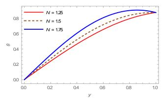
**Figure 12-**Influence of *N* on Temperature  $\theta$  for  $\omega = 1$ , Pe = 0.7, t = 0.5
