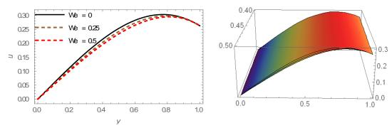
**Figure 11-**Velocity profile for We with  $\omega = 1$ , N = 1, Re = 1, Pe = 1, M = 1, N = 1, N
