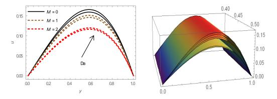
**Figure 2**-Velocity profile for Da and M with  $\omega = 1$ , N = 1, Gr = 1, Re = 1, Pe = 1,  $\lambda = 1$ , We = 0.05, t = 0.5 in Poiseuille flow.
