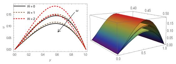
**Figure 5-**Velocity profile for  $\omega$  and N with Re = 1, Pe = 1, M = 1,  $\lambda = 1$ , Gr = 1, Da = 0.8, We = 0.05, t = 0.5 in Poiseuille flow.
