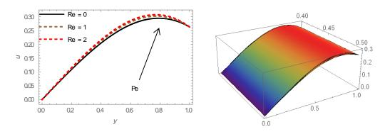
**Figure 9-**Velocity profile for Re and Pe with  $\omega = 1$ , N = 1, M = 1,  $\lambda = 1$ , Ge = 1, Da = 0.8, We = 0.05,  $V_0 = 0.3$ , t = 0.5 in Couette flow.
