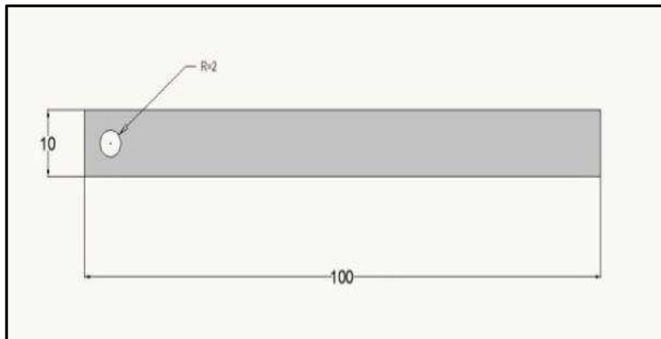
**Figure 3-** Fatigue specimen according to the machine's manual [18] (all dimensions are in mm).
