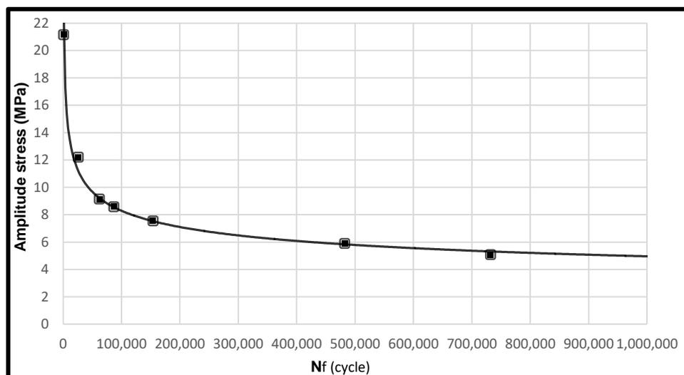
**Figure 4-** SN curve of polyester\ Al powder without any treatment.
