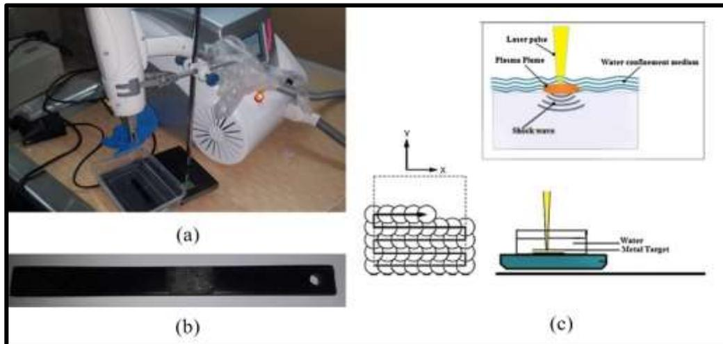
**Figure 1**(a)-Q-switched Nd-Yag laser pulse, (b) Fatigue specimen when treated by confined laser peening and (c) Schematic diagram and basic principle of laser peening [16]
