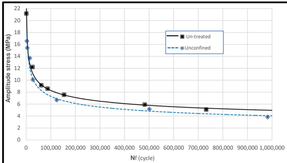
**Figure 5-**Comparison between SN curves of polyester/Al powder without and with treatment by water confined laser peening.
