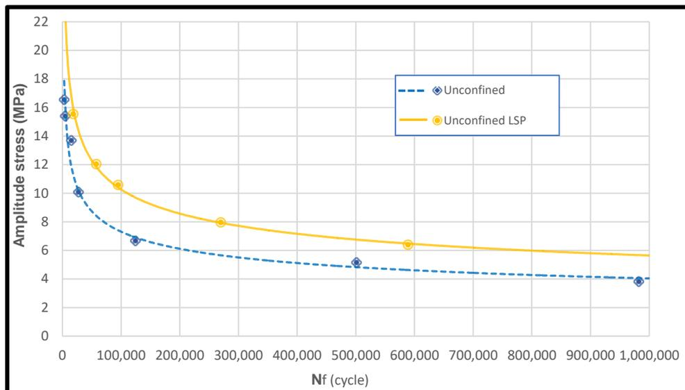
Figure 7-Comparison between S-N curves of polyester\ Al powder after treatment by unconfined and confined laser peening.
