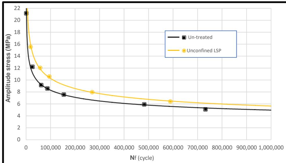
Figure 6-Comparison between S-N curves of polyester\ Al powder without and with treatment by unconfined laser peening.
