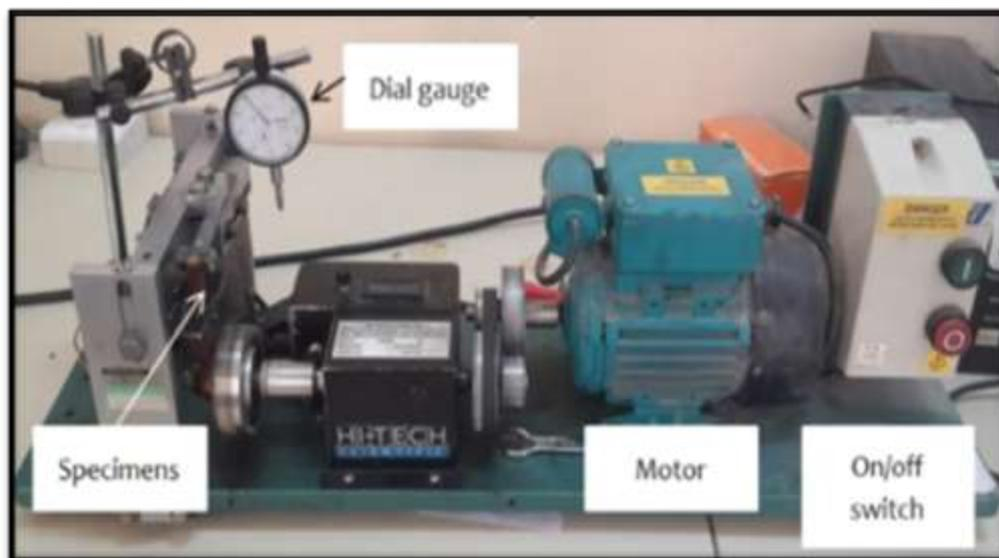
**Figure 2-** Bending- alternating fatigue device HSM20.
