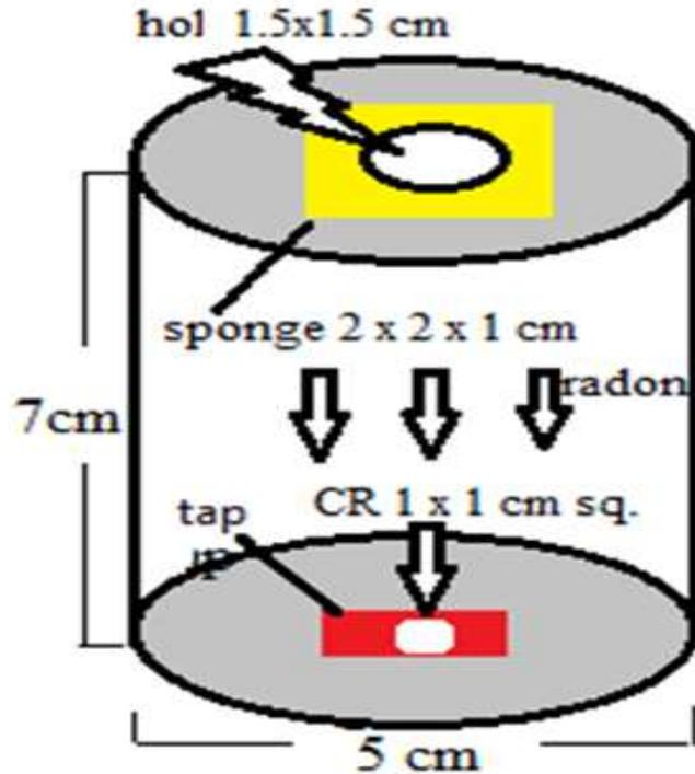
Figure 1- Radon monitors “Can technique”.
