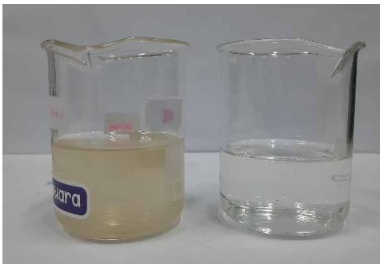
Figure 14: Inlet wastewater before (left) and after (right) AC-CBW adsorbent application
