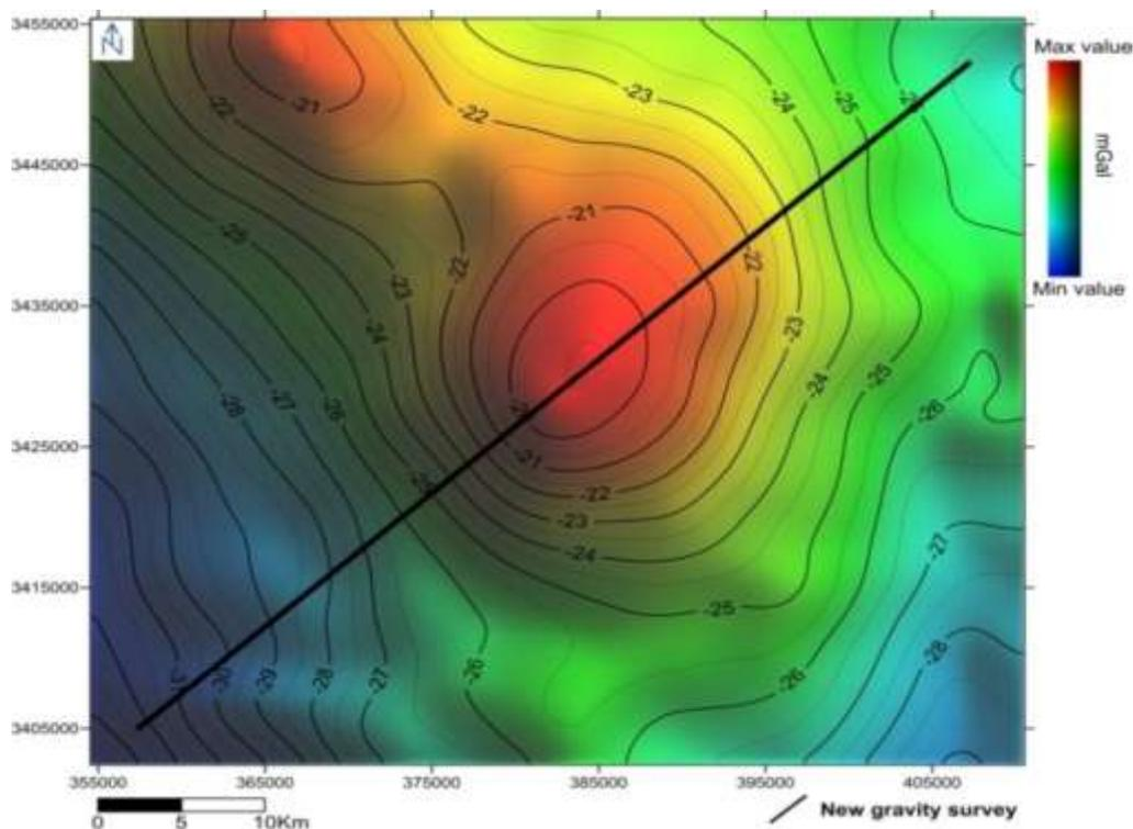
**Figure 5-**Gravity Bouguer map shows the positive anomaly which takes its axis N- S,the axis drift at the northwest of the study area to NW- SE , the new profile survey is passing at the dip of the general anomaly and covered it.
