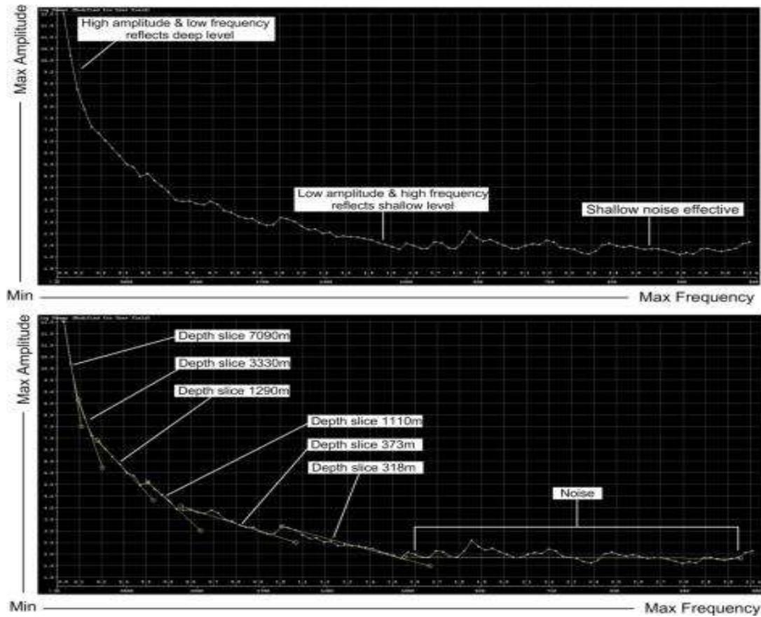
**Figure 12-**Power spectrum of the new gravity profile, shows the wave number of high/ low amplitude and frequency. Present in gravity depth slices levels and shallow noise effective.
