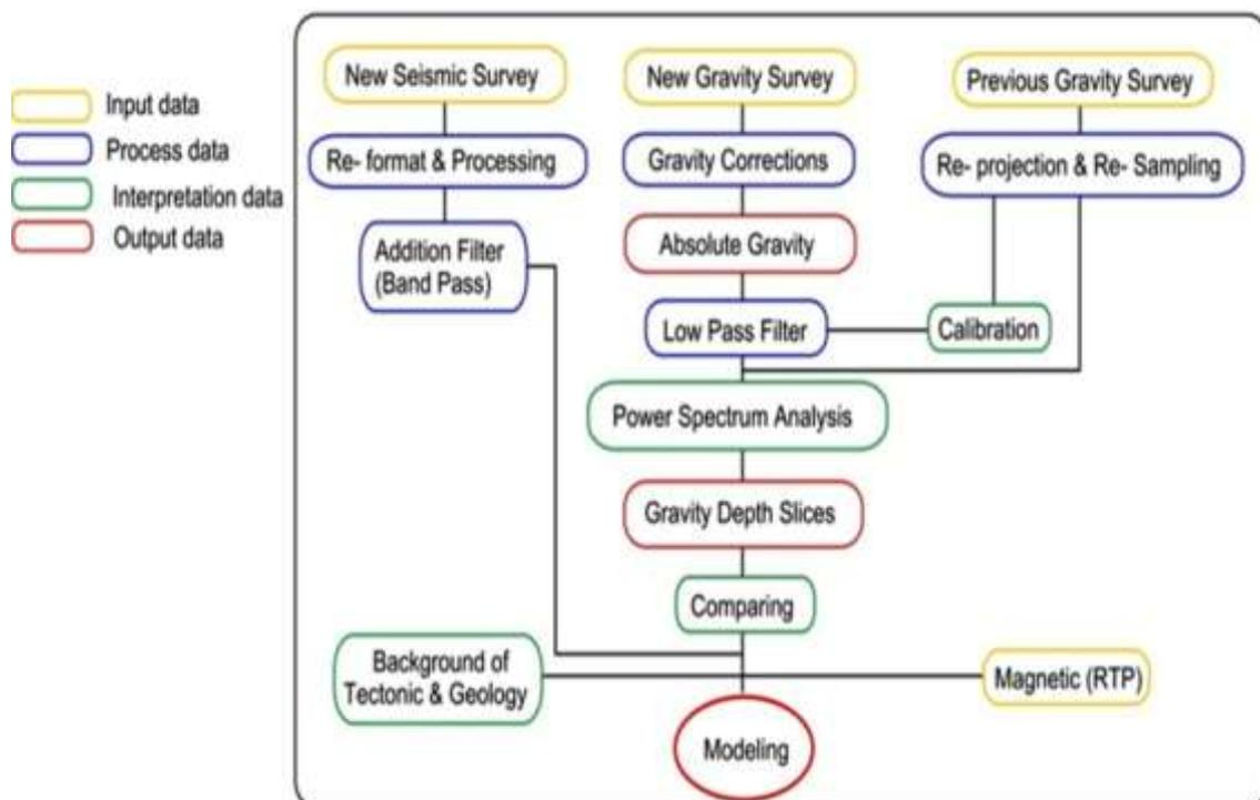
**Figure 11**-Flow chart of current geophysics integration based on (input data, processing, interpretation and output data).
