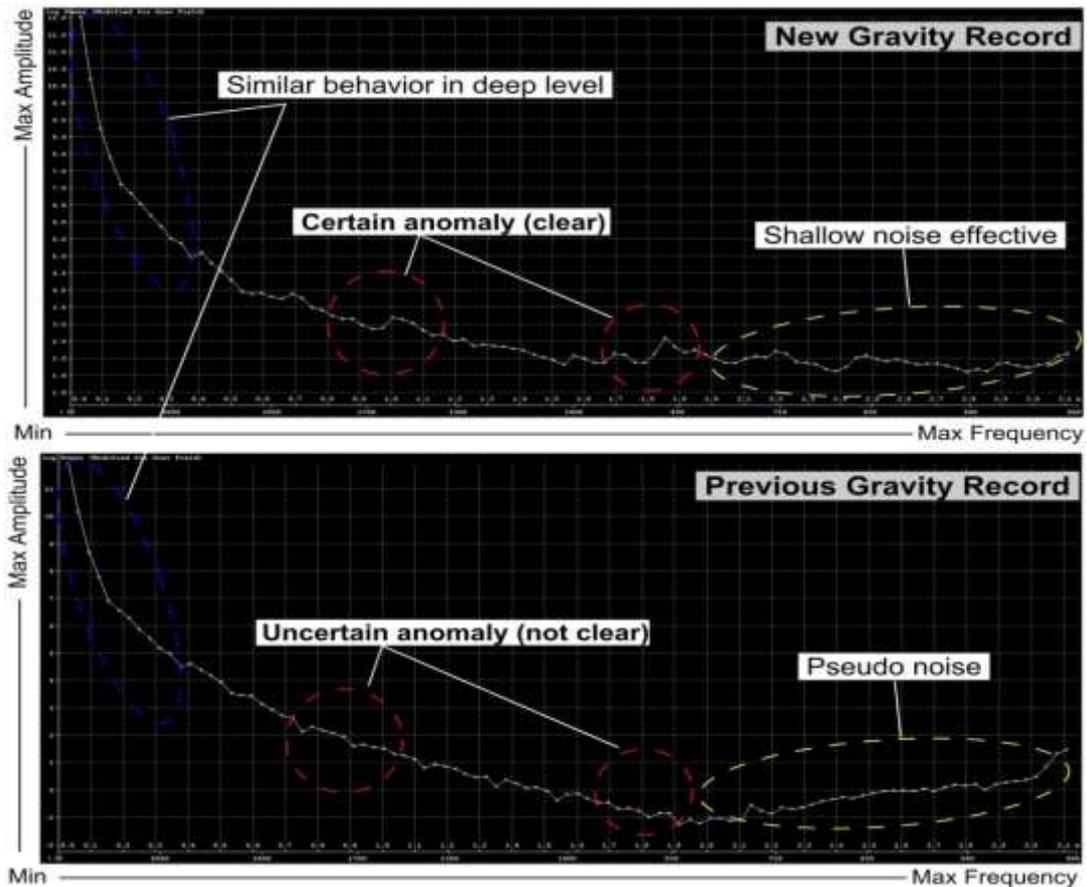
**Figure 14-**Comparison between the new and previous gravity profile in power spectrum domain, showing the similar behavior in deep level (indicator in blue), new gravity profile obtain better details in shallow levels (indicator in red), the shallow noise effective (indicator in yellow) seems pseudo noise in previous gravity profile.
