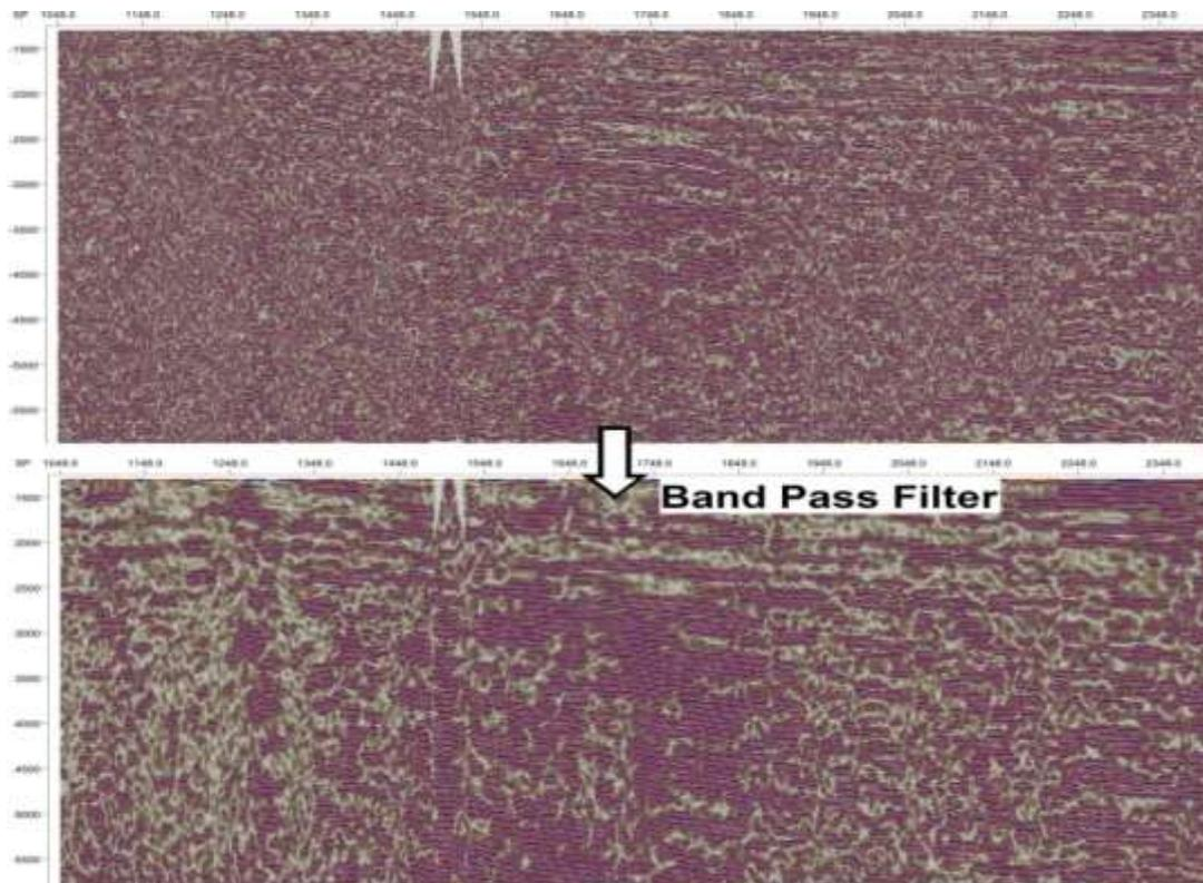
**Figure 10**-New Seismic section (7Gn- 16) shows the enhancement of features after applying the band pass frequency filter.
