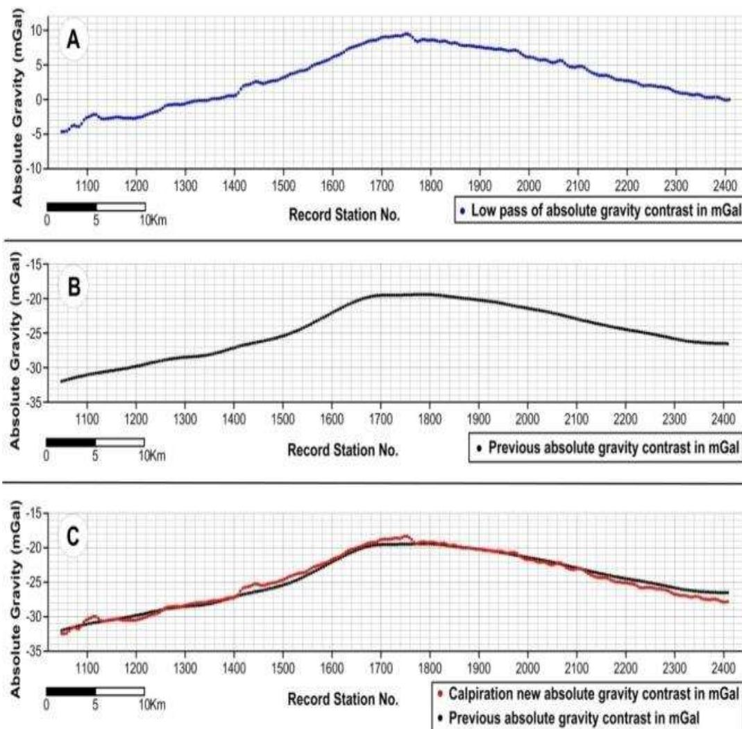
**Figure 6-** Shows the calibration of the gravity values between the two surveys. A- Blue profile is the new gravity values contrast, range from (-4.64 to 9.22) mGal. B- Black profile is the previous gravity values contrast, range from (-31.6 to 19.4) mGal. C- Calibration new gravity values contrast (Red profile) at the previous gravity survey.
