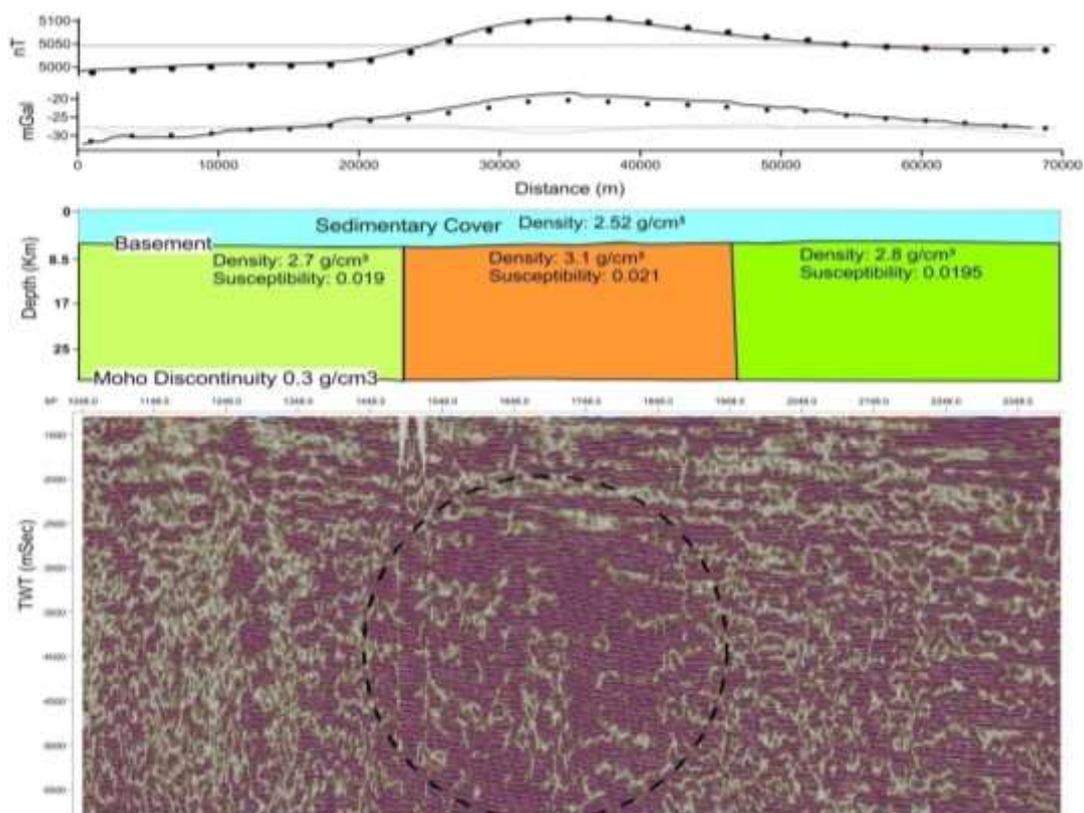
**Figure 16**-Supposed simple deep modeling at Moho discontinuity comparing with seismic section filtered (Band pass), shows the effective of higher gravity & magnetic anomaly due to higher density and magnetic sensitivity in deep level.
