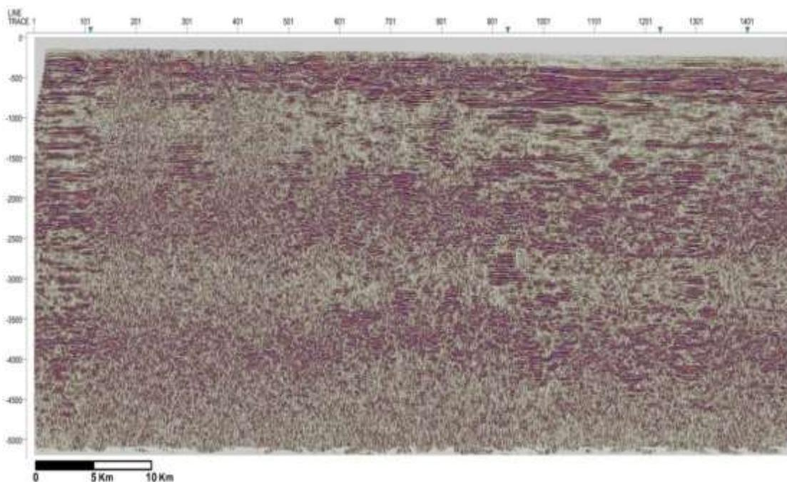
**Figure 8-**Previous seismic section (1979) in time domain of line 1Gn- 32 which corresponds the location of gravity survey, [8].
