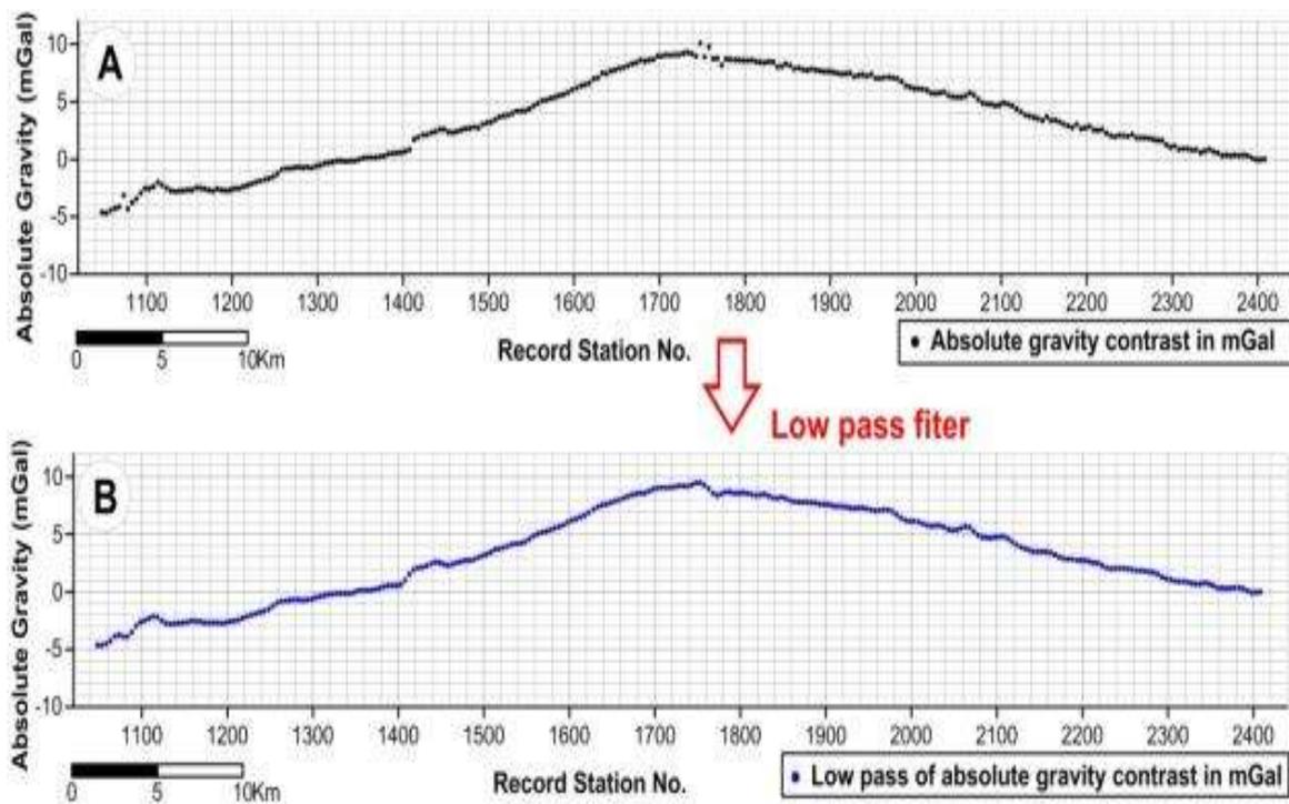
**Figure 4-**Applying simple low pass filter to gravity observed of datum (200m ASL), using software (GeoSoft- Oasis Montaj version 8.4). A- Profile shows some noise in start and mid of path at station. B- Profile shows remove the noise after applied simple low pass filter.
