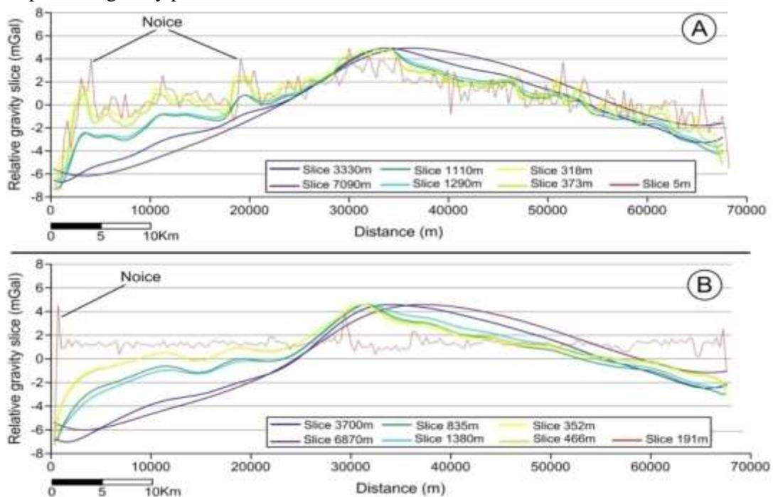
**Figure 15-**Compare the domination slices of new gravity (A) and previous gravity profile (B): (A, B) are similar behavior in deep level (indicator in purple & blue curve). (B) Shallow noise effective (indicator in light red curve) seems pseudo noise.
