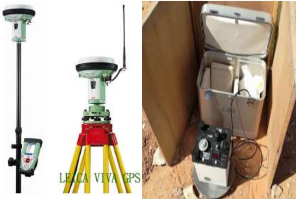
Figure 3-The (LEICA VIVA GPS) and the gravimeter (LACOSTE and ROMBERG- G. 532) used in the field survey.
