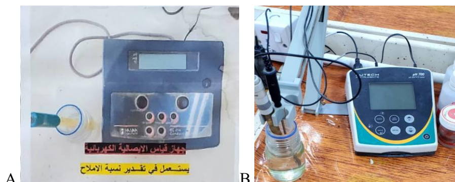
Figure 2: (a) Electrical conductivity meter, (b) pH meter.
