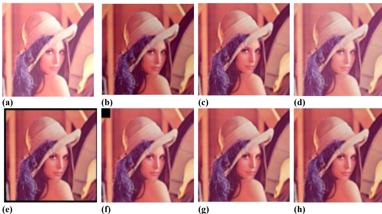
Figure 10: Attacked Watermarked Images: (a) image brightening, (b) darkened image, (c) histogram Equalization, (d) Gamma Corrected Bright, (e) cropped border (20px each side), (f) cropped image (10%), (g) Multiplicative noise (0.03), (h) Gaussian noise (0.1)
