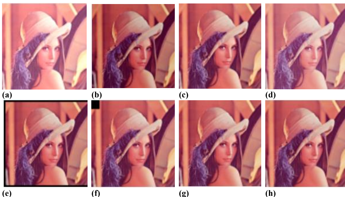
Figure 10: Attacked Watermarked Images: (a) image brightening, (b) darkened image, (c) histogram Equalization, (d) Gamma Corrected Bright, (e) cropped border (20px each side), (f) cropped image (10%), (g) Multiplicative noise (0.03), (h) Gaussian noise (0.1)
