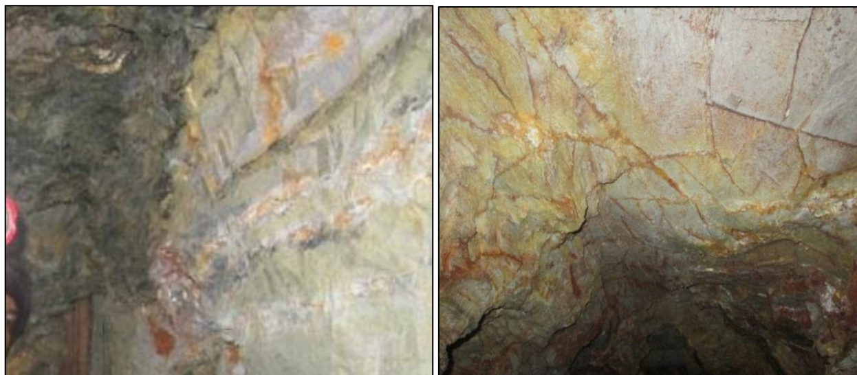
Figure 7: A. Quartz Vein with a 40-50 cm thickness and crustiform banding texture (alternation of quartz and sulfide). B The mineralised zone in the shaft shows vein stockwork that indicates an alteration in grey, greenish, yellow, and white colours (indications of chlorite, quartz, and silicic)
