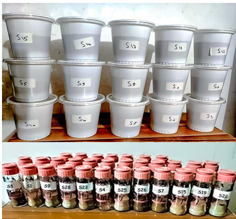
Figure 2: Preparation of soil samples for gamma analysis and radon concentration measurement.
