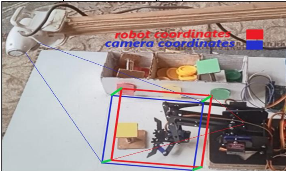
Figure 4: The workspace area of the system (highlighted by a square box) the red square is exactly above the blue one.
