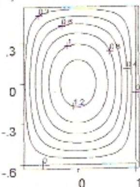
Fig.(37),axial velocity for \beta=1,k=1.77,L=0.01,\tau=0.39
