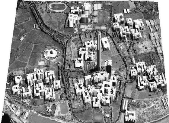
Figure 7 : The 3-D photo image merge with final DEM using universal kriging technique
