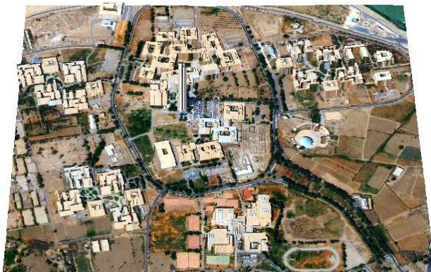
Figure 8 : The 3-D photo image merge with final DEM by nearest neighbor technique.
