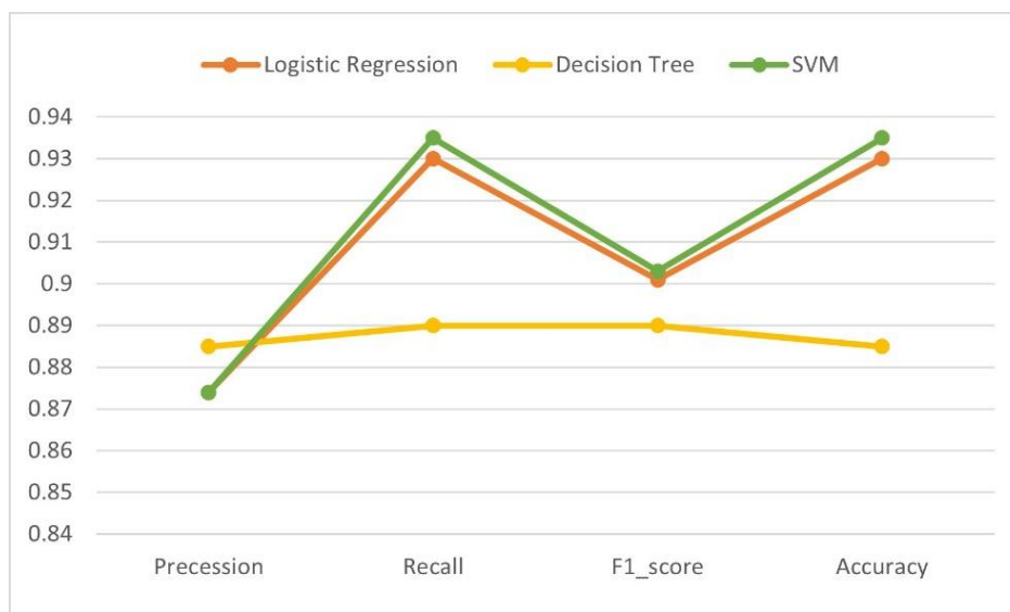
Figure 2: Results of logistic regression, decision tree, and SVM in terms of (precision, recall, F1_score, and accuracy)
