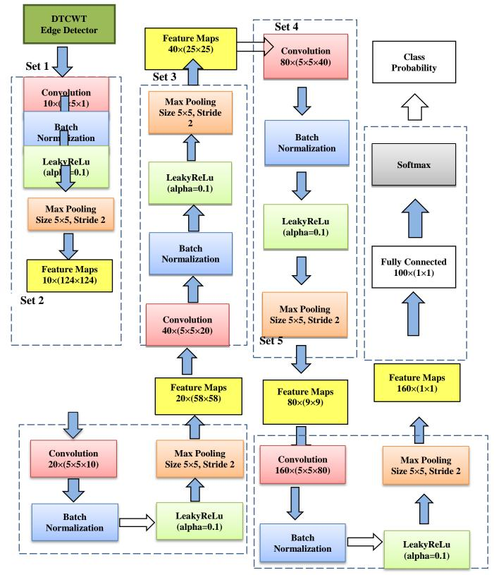
Figure 1-Convolution Neural Network of system
