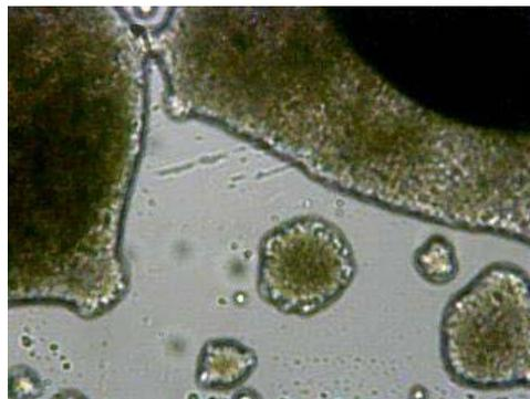
**Figure 10: Nematic texture of compound (11)<sub>a</sub> at 185°C.**
