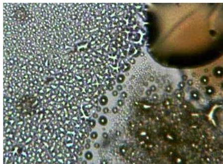
**Figure 8: Nematic texture of compound (11)<sub>b</sub> at 205°C.**
