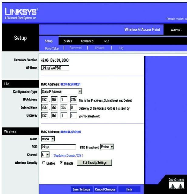
Figure 3: Basic Setup Screen to Change SSID and Default IP
