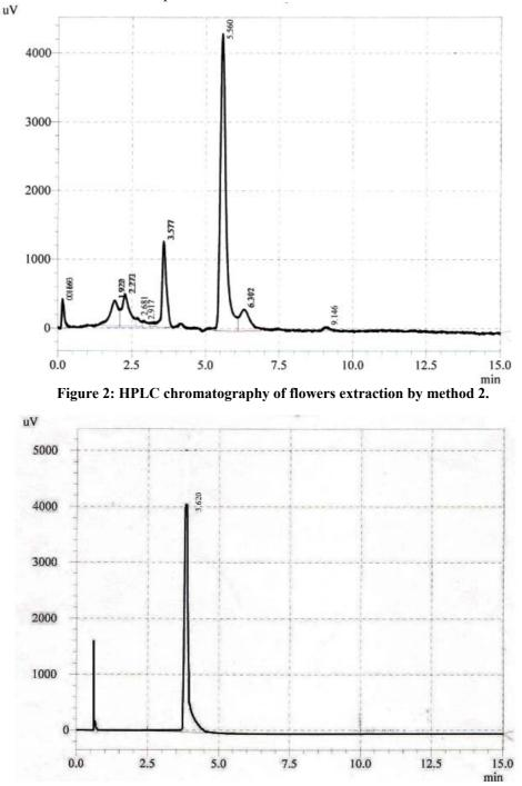
Figure 3: HPLC chromatography of standard pyrethrin I.
