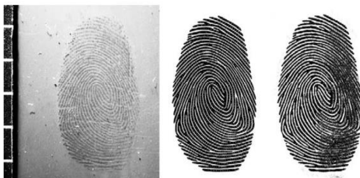
Figure 1: Deposited fingermark (left), final image (middle) after processing with Adobe Photoshop1 CS2, and capture (right) taken from the final fake fingerprint built with glue from an indirect cast printed on an acetate sheet [12].
