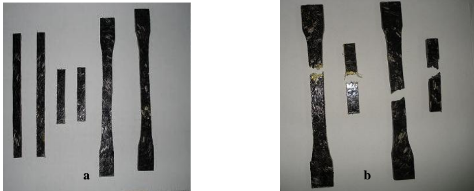
Figure 2: Samples of flexural, impact and tensile test (a) before and (b) after tests
