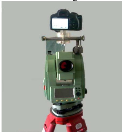
Figure 4- Leica Total Station System With Cannon Camera.
