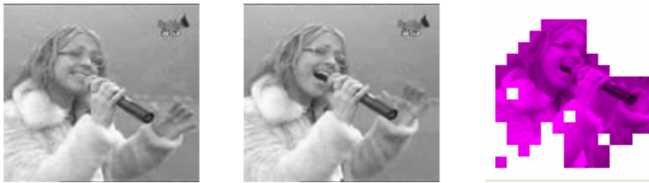
Figure 7- Represent Reconstruction Images (I) And (P) And Block Different When We Apply (NTSS) Used (MAD) Criteria With Thr.4
