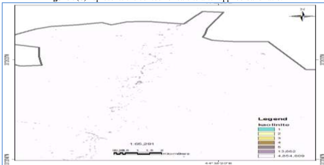
Figure 6(a) -the Kaolinite can be observed at varying rates depending on the geological characteristics of the area. The formula was [\text{band4} / \text{band5}] [\text{band8} / \text{band6}] , [11].
