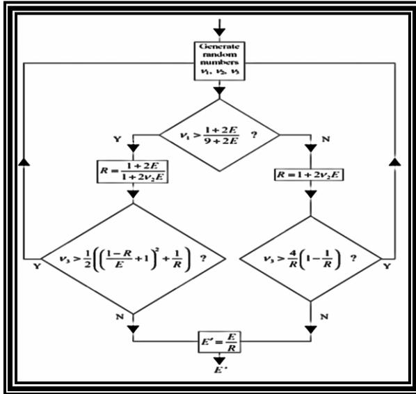
**Figure 2-** method for random sampling of the Klein – Nishina distribution by Kahn method [6].
