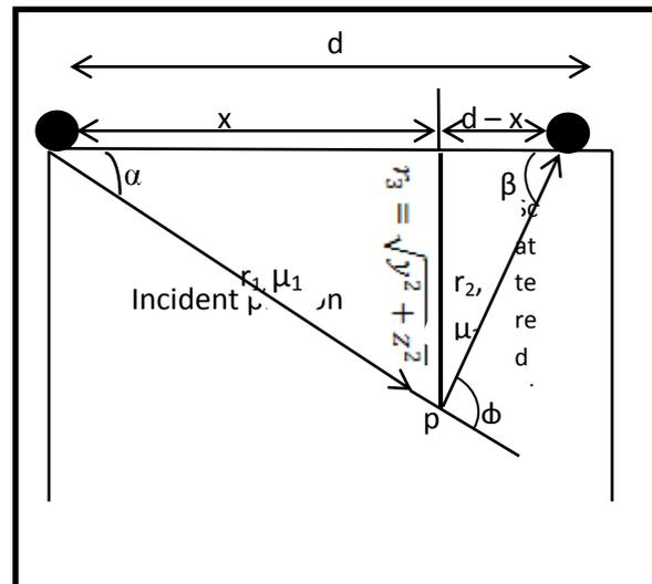
Figure 1- Basic geometry for a Compton backscatter densitometer
