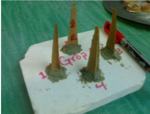
Figure 4(a)- Choosing samples of refractoriness test before firing
