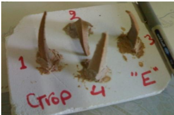
Figure 4(b)- Choosing samples of refractoriness test after firing
