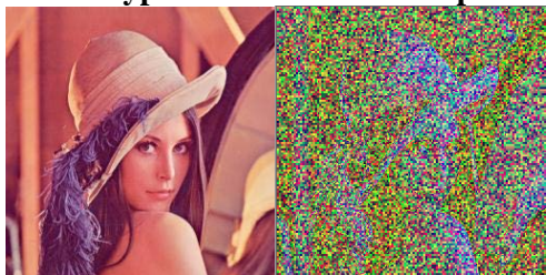
Original image Image size 256*256 Encrypted image prime=257 Size of mask =17*2
