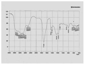
Figure 1- FTIR spectra of Poly acrylic acid.
