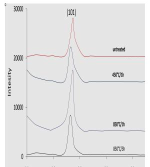
Figure 2- Illustration of X-ray line broadening for calcinated kaolin.
