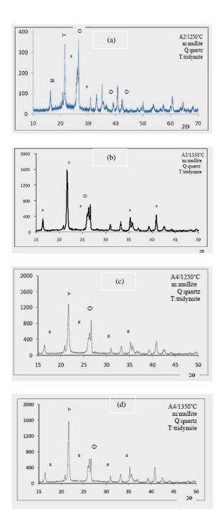
Figure 5- (a-d) XRD patterns for the fired samples A2 and A4 at 1250°C and 1350°C for two hours
