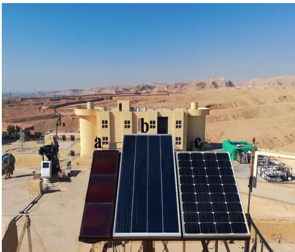
Figure 1: Field test equipment for three Si modules: (a) amorphous module, (b) poly-crystalline module, and (c) mono-crystalline module
