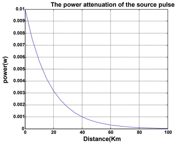
**Figure 6** This curve represents the power of the source pulse travelling through an optical fiber of 100 km length (distance).
