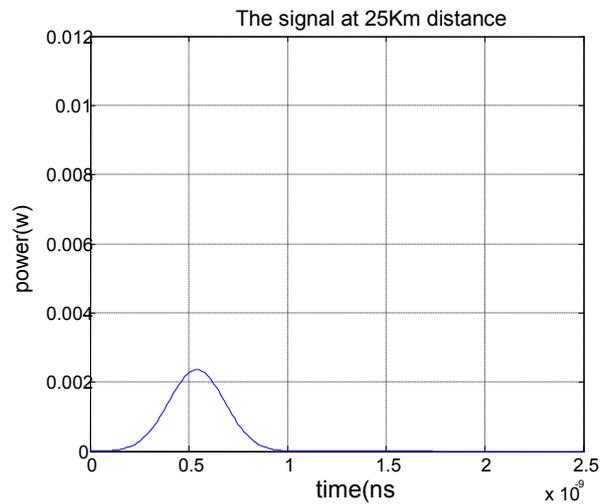
**Figure 4** The source signal at 25km distance through the optical fiber where the puls is 2.21 mW.
