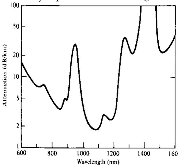
**Figure 1-** Attenuation –versus –wavelength curve
