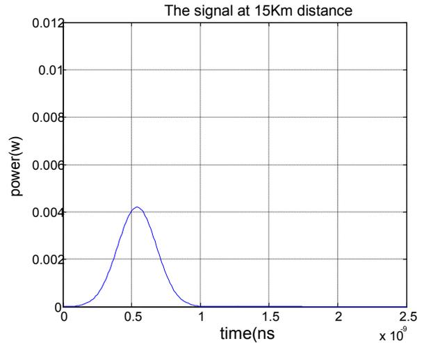
**Figure 3** This signal represents the shape of source at 15 km distance. The effect of attenuation is shown on the pulse amplitude which was 4.217 mW.
