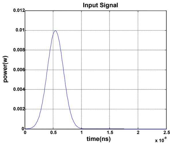
**Figure 2** This Pulse represents the Input signal to the Optical Fiber from 10 mW Laser source of 1ns duration.
