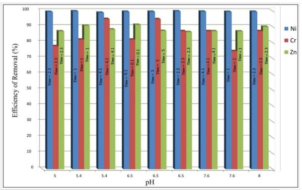
Figure 2- Effect of pH on three heavy metals removal efficiency by corn cobs.
