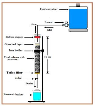
Figure 1- Schematic presentation of the experimental column.
