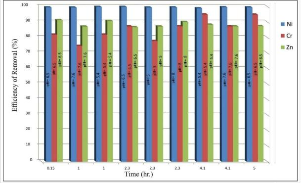
Figure 3- Effect of contact time on three heavy metals removal efficiency by corn cobs.
