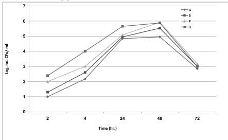
**Figure 4-** Relationship between time and log.no. of *A.hydrophlia*.(*DW* isolate) on four solid surface at 37°C and pH 7. stainless steel (S), galvanized iron(G) adhered cells, polyvinyl chloride (P) and unplasticised polyvinyl chloride(U)
