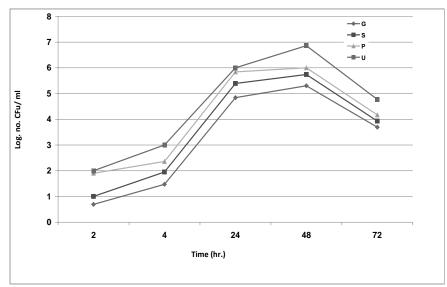
**Figure 9**- Relationship between time and log.no. of *A.hydrophlia* (RW) isolate on four solid surface at 40°C adhered cells stainless steel (S), galvanized iron(G), polyvinyl chloride (P) and unplasticised polyvinyl chloride(U)
