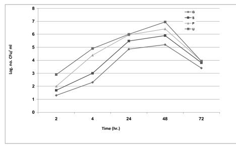
**Figure 5-** Relationship between time and log.no. of *A.hydrophlia* on four solid surface at  $37^{\circ}C$  and pH 7. stainless steel (S), galvanized iron(G) (*RW* isolate) adhered cells, polyvinyl chloride (P) and unplasticised polyvinyl chloride(U)
