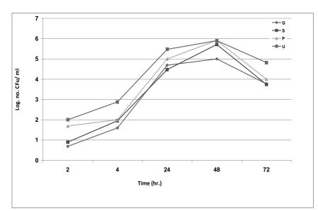
**Figure 8-** Relationship between time and log.no. of *A.hydrophlia* A.(*DW* isolate) on four solid surface at 40°C adhered cells stainless steel (S), galvanized iron(G), polyvinyl chloride (P) and unplasticised polyvinyl chloride(U)
