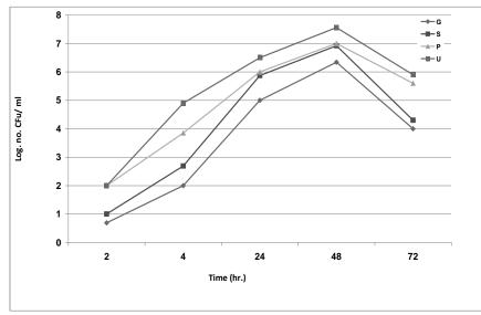
**Figure 6-** Relationship between time and log.no. of *A.hydrophlia.(DW* isolate) adhered cells on four solid surface at 5 °C. stainless steel (S), galvanized iron(G), polyvinyl chloride (P) and unplasticised polyvinyl chloride(U)
