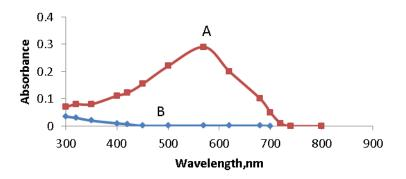
**Figure 2-** Absorbance spectra of thymol  $(4\mu g \text{ mL}^{-1})$  treated as described under procedure above and measured against blank(A), The reagent blank contains all components except Thymol measured against distilled water(B).
