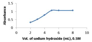
**Figure 3- Effect** of the volume of NaOH( 0.5M ) for determination of Thymol (8µg.mL<sup>-1</sup>).
