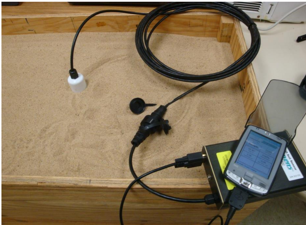
Figure 3: In situ dielectric constant measurements by Steven's Soil Sensor
