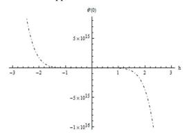
**Figure 3-** 3th-order of approximation h curve for  $\theta'(\eta)$
