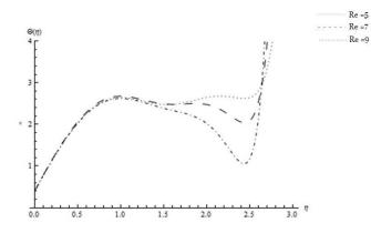
Figure 9- Heat distribution with , , M = 1, h = -0.2, Kn = 0.1, W = 1, Pe = 9 , Br = 6 . Re = 5,7,9.
