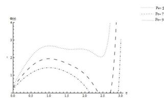
Figure 13- Heat distribution with , M = 1, h = -0.2, Re = 7.1, W = 1, kn = 0.1 , Br = 6 . pe = 5, 7, 9.
