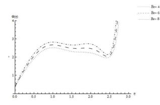
Figure 12- Heat distribution with M = 1, h = -0.2, Re = 7.1, Kn = 0.1, Pe = 9, W = 1. Br = 4,6,8.
