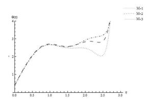
Figure 8- Heat distribution with, Re = 7, h = -0.2, Kn = 0.1, W = 1, Pe = 9, Br = 6. M = 1, 2, 3.
