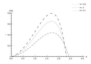
Figure 7- Velocity distribution with , M = 2, h = -0.2, kn = 0.1, Re = 7. W = 0.5, 1, 0.2
