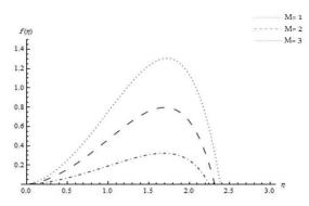
Figure 4- Velocity distribution with, Re = 7, h = -0.2, W = 1, kn = 0.1. M = 1, 2, 3.
