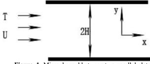
Figure 1- Microchannel between two parallel plates
