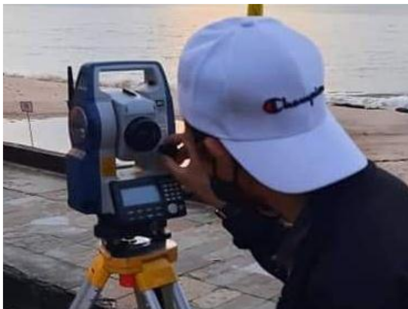
Figure 1: Sokkia Total Station CX 103 During the Observation of the new crescent Moon of Zulkaedah 1443[15][16].
