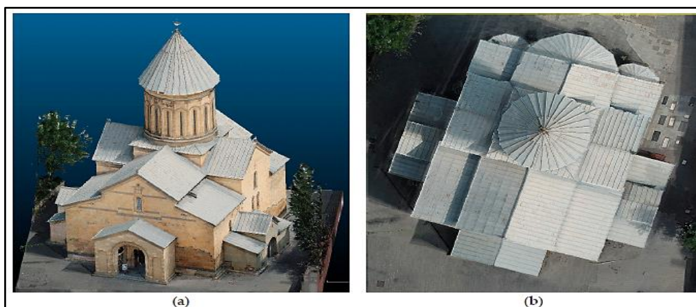
Figure 8: The final 3D model is based on combined photogrammetry and laser scanning. [97]
