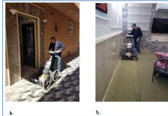
Figure 5: The GPR survey, a. outside the building, b. inside the building.
