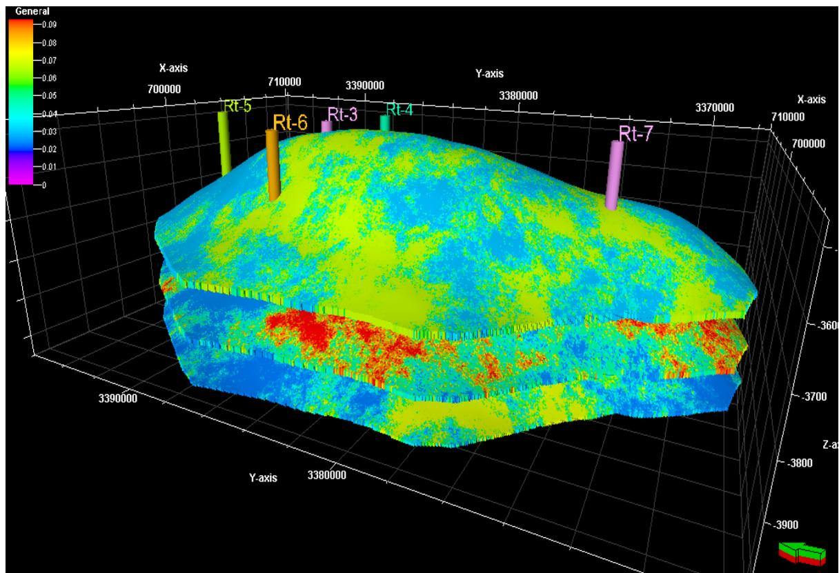
Figure 5-The porosity model of the three reservoirs (YR-A, YR-B, YR-C) in Ratawi field.
