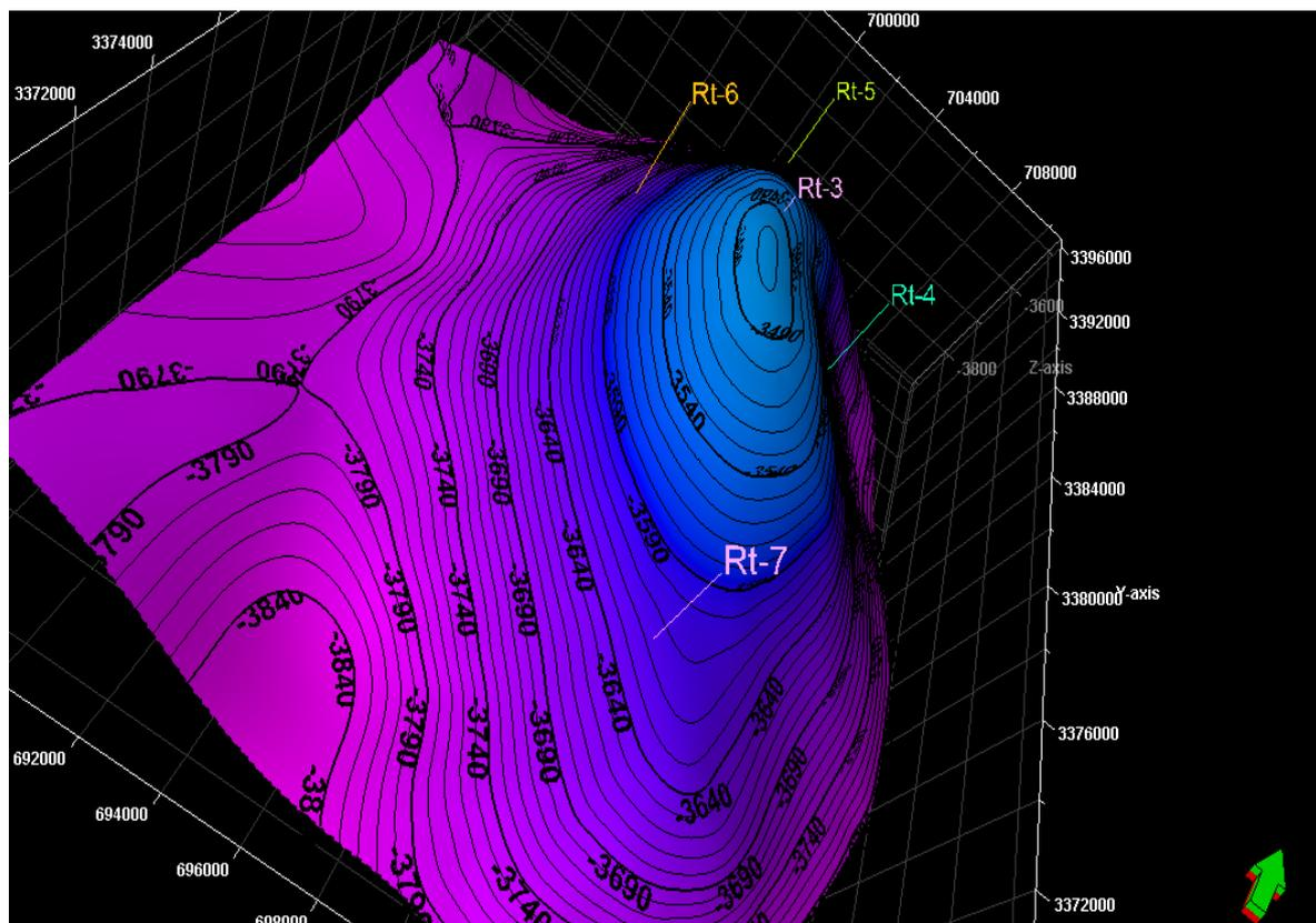
Figure 4- structural contour map on top of the Yamama Formation in Ratawi field.
