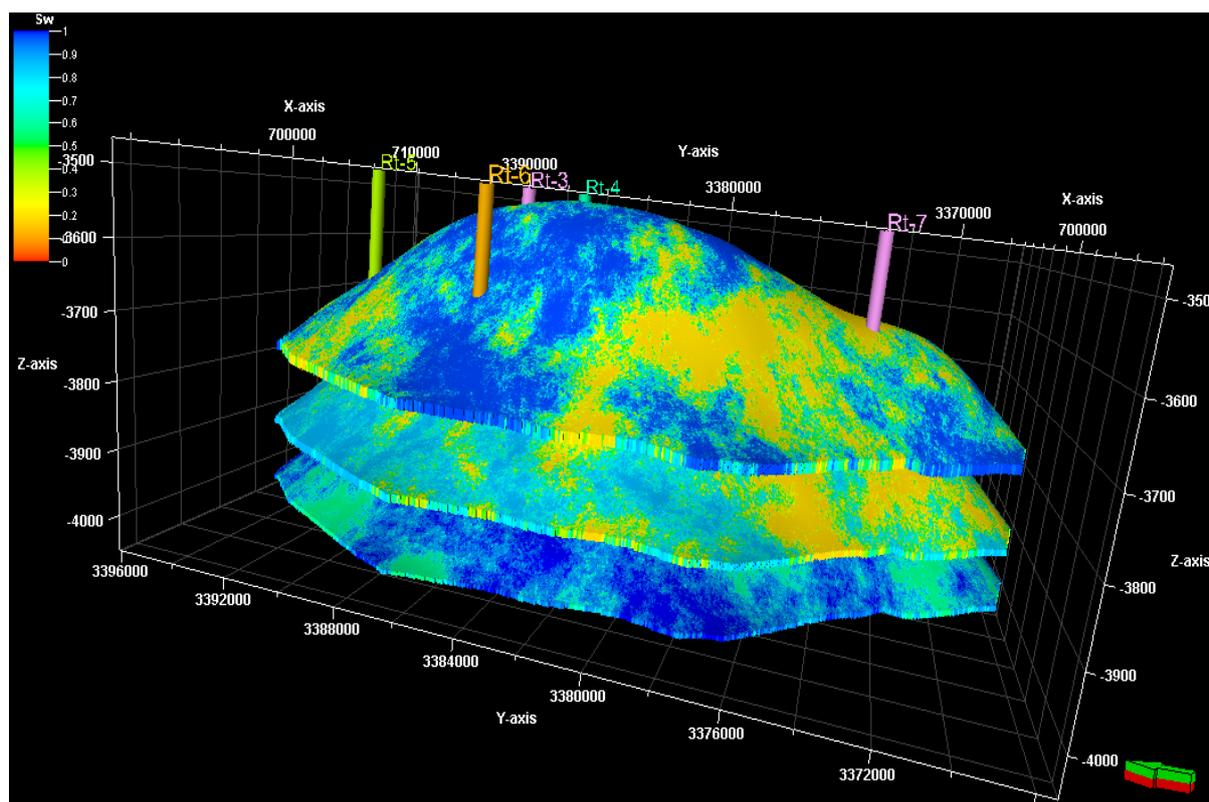
Figure 6- The water saturation model of the three reservoirs together (YR-A, YR-B, YR-C) in Ratawi field.
