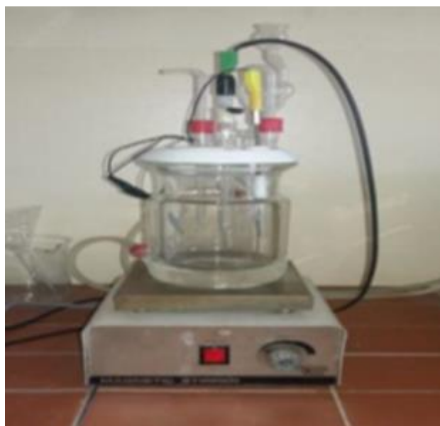
Figure 3: The corrosion cell used during the current study
