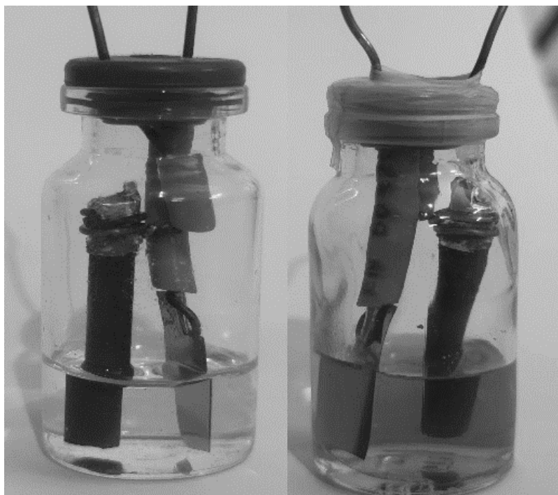
Figure 2: Illustration of a TiO 2 NTAs-graphite electrochemical cells
