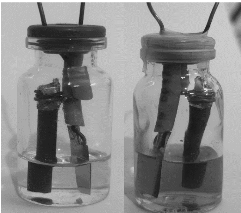
Figure 2: Illustration of a TiO 2 NTAs-graphite electrochemical cells
