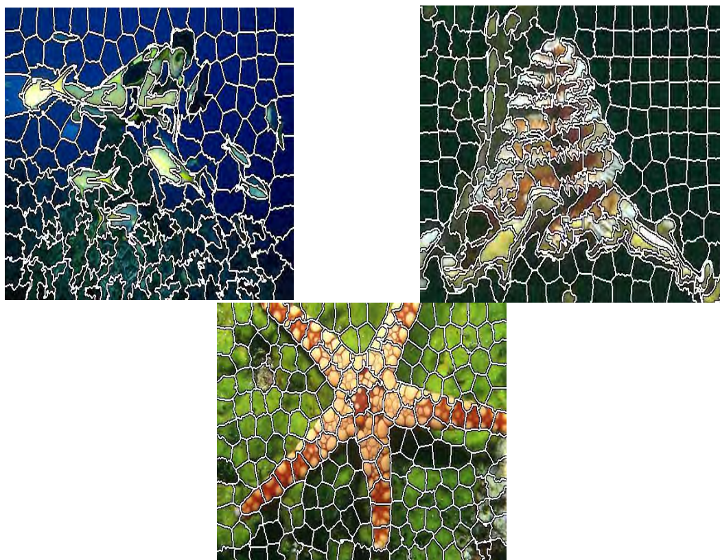
Figure 1 -Represents the output of SLIC algorithm with a constant compactness Factor for all superpixels [7].
